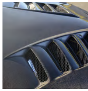
Eight individual air vents protrude from the carbon fibre bonnet to maximise air flow
